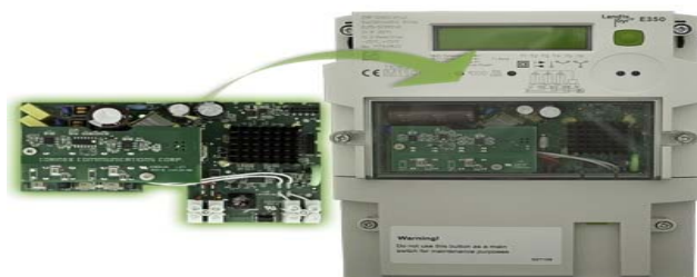
Figura 41. Smart Meter Communication Module L&G CXM-SG200-MDL.
