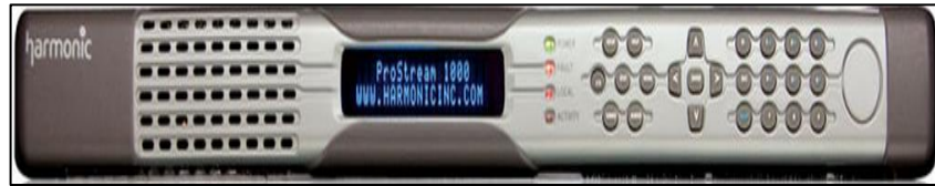
Figura 27: Multiplexor Harmonic ProStream 1000 Fuente: (Harmonic, Inc)
