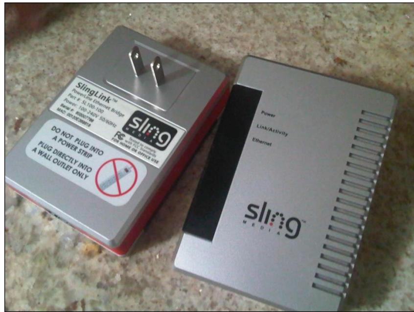
*Figura IV.2 CPE “SlingLink Power Line Ethernet Bridge” (Panel Frontal y Posterior)*
