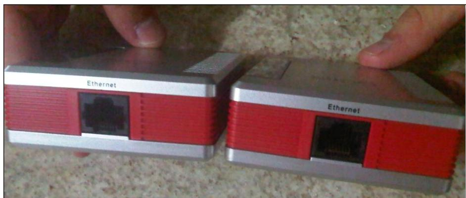
*Figura IV.1* Dispositivo CPE “*SlingLink Power Line Ethernet Bridge*”
