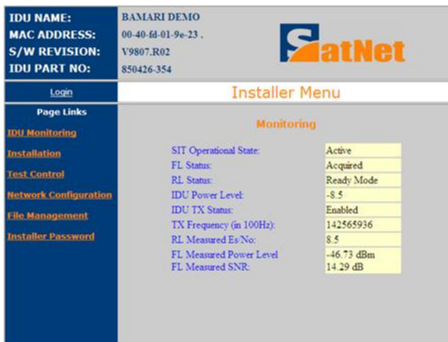
Figura 28 Installer Menu (cadena 1)
