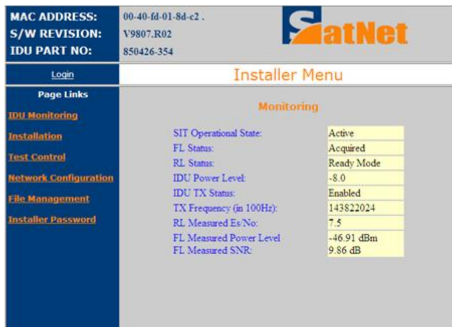
Figura 27 Installer Menu (cadena 2)
