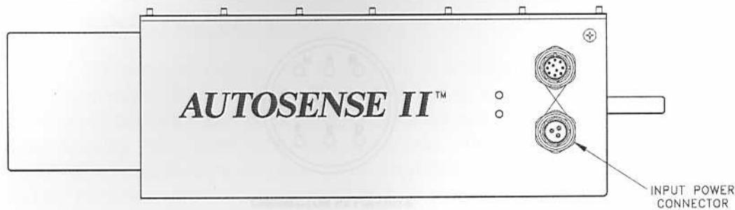
**Figure 2-2. Power Cable Connection.**
