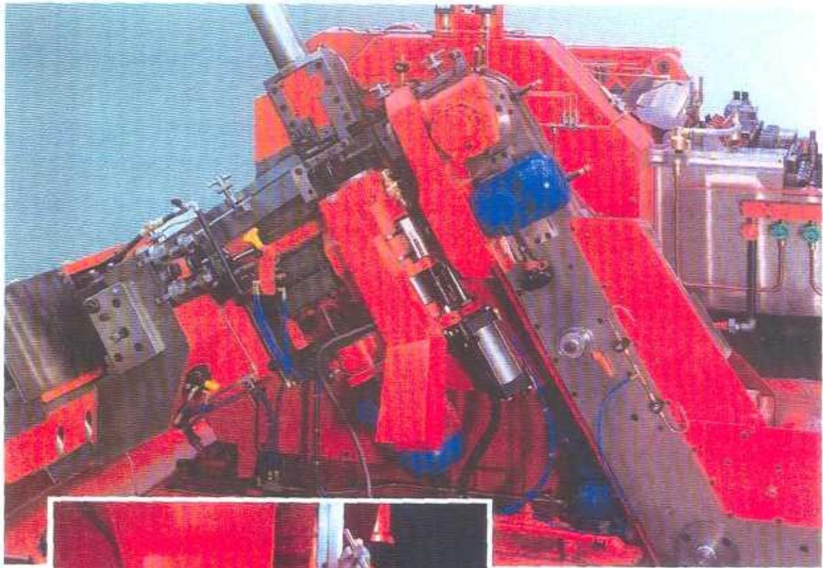
*Elevator with pointing and threadbusting stations.*
